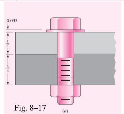
From Table A-32, the thickness of a standard  $\frac{1}{2}$  N plain washer is 0.095 in. (a) As shown in Fig. 8-17b, the frusta extend halfway into the joint the distance
