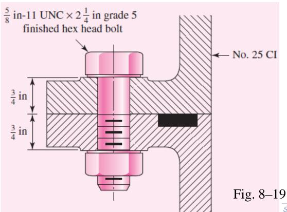
(a) The grip is l = 1.50 in. From Table A–31, the nut thickness is  $\frac{35}{64}$  in. Adding two threads beyond the nut of  $\frac{2}{11}$  in gives a bolt length of
