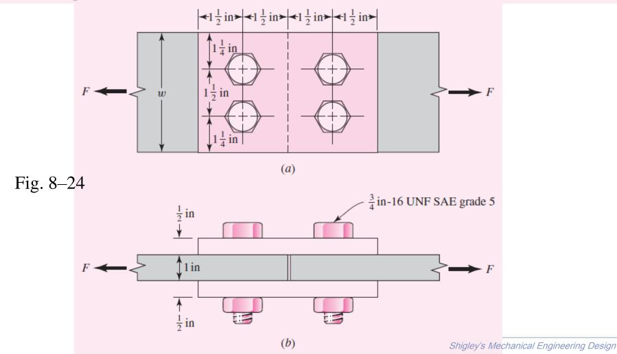
From Table A–20, minimum strengths of  $S_y = 54$  kpsi and  $S_{ut} = 64$  kpsi are found for the members, and from Table 8–9 minimum strengths of  $S_p = 85$  kpsi and  $S_{ut} = 120$  kpsi for the bolts are found.
