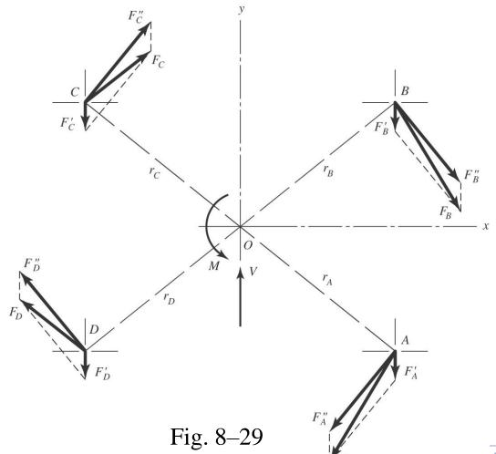
The primary shear load per bolt is
