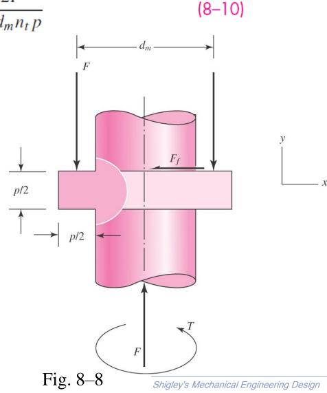
Bending stress at root of thread,
